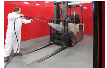
User safety features: non-slip diamond plate deck with a level covered grate
